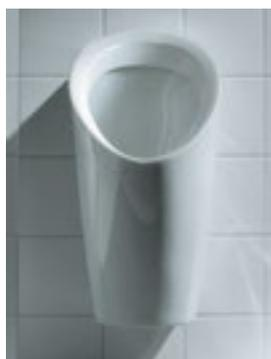
The LAUFEN Lema 0-litre urinal saves water and money. It operates without water and does not require a water shut-off device or electricity to keep the drain closed. The urine itself helps to keep gases sealed in and to prevent their escape. The principle behind this "trap" is known in the chemical industry as the Erlenmeyer flask.
