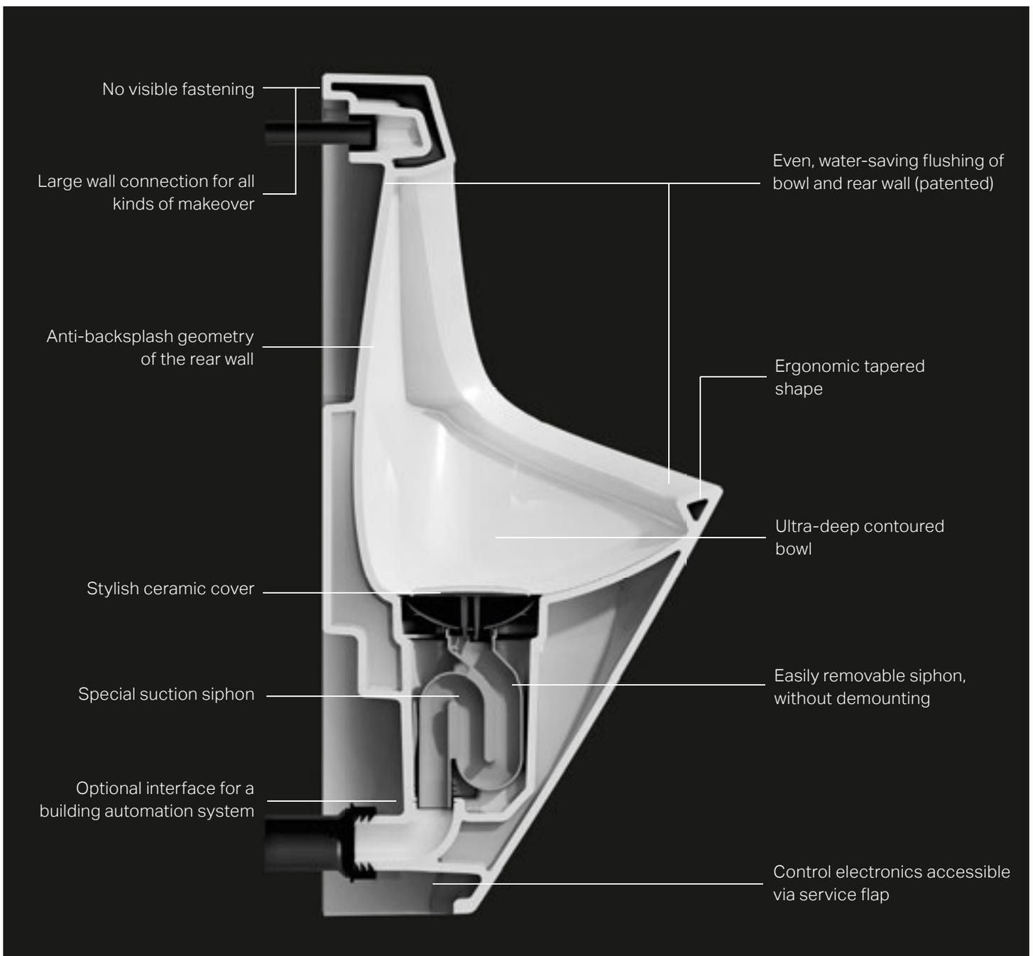
LAUFEN urinals are revolutionising the upkeep and maintenance of public sanitary facilities. Up till now, urinals often had to be completely disassembled when replacing their siphons. ANTERO and LEMA allow you to release and pull the siphon out easily using a special key.
