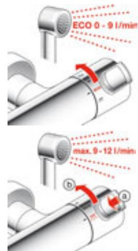
Regulate the water flow at the turn of a hand. Use the Eco button to easily save more water (see illustration 5). By pressing the stop button you leave the ECO range and the water runs at full flow (see illustration 6).
