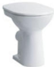
Floorstanding WC ,comfort', washdown, with flushing rim, outlet horizontal, sitting height 450 mm (without WC seat)
