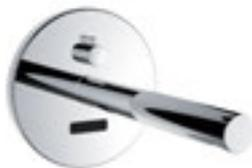
Concealed basin mixer, with electronic control, manual temperature setting, projection 200 mm, fixed spout, battery operated (6V) / mains operated (230V), with Bluetooth adapter
